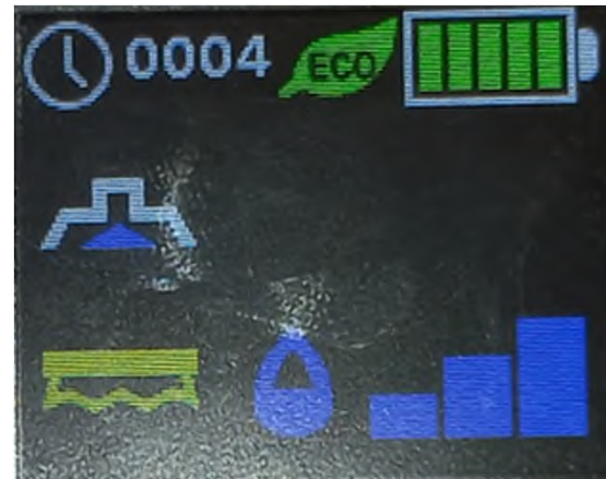
if a working tool is shown in YELLOW it is not released
